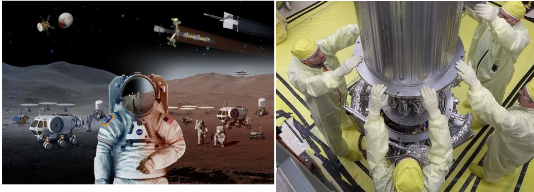
NASA and NNSA engineers lower the wall of the vacuum chamber around the Kilowatt Reactor Using Stirling Technology (KRUSTY system). The vacuum chamber is later evacuated to simulate the conditions of space when KRUSTY operates. Credits: Los Alamos National Laboratory
